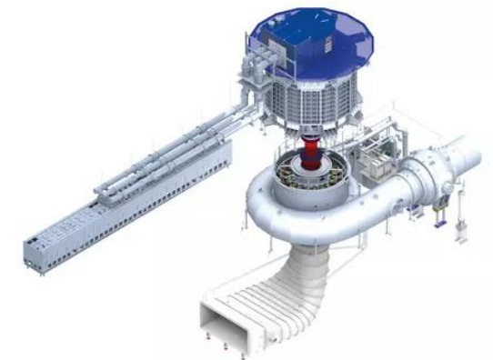
VARIBLE SPEED UNIT Credit – Voith Hydro 780 MW Frades II PSH Portugal
